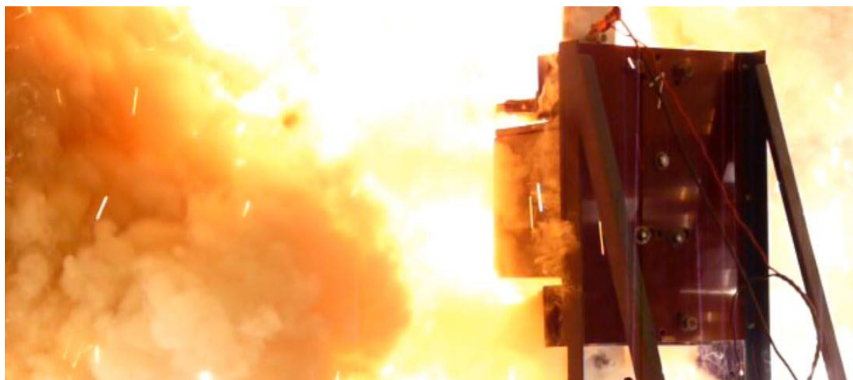
A searing plasma and gas cloud is produced by an electrical arc in a testing box
